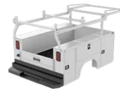
UTILITY RACK 1,000 lb. capacity - forklift loadable
