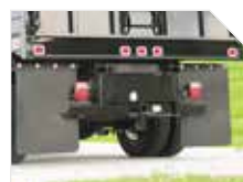
COMBINATION CLASS V HITCH AND ICC BUMPER
