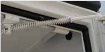
NEOPRENE DOOR SEALS protect compartments from the weather
