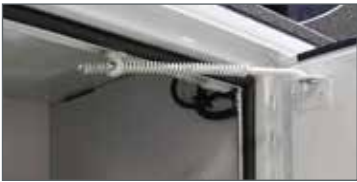
DOUBLE-SPRING OVER-CENTER RETAINER on vertical compartment doors eliminate involuntary swing
