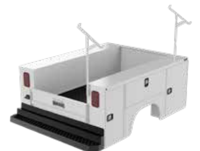
SIDE MOUNT LADDER RACK 150 lb. capacity
