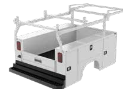
UTILITY RACK 1,000 lb. capacity - forklift loadable
