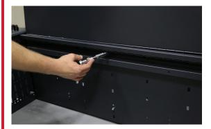
Open the door hinge and place the underside of the door hinge over the top/front edge of the upgradeable shelf. Line up the holes in the door hinge with the holes along the front of the shelf.
