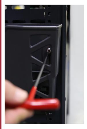
Determine the desired location to mount the storage pocket. Secure the storage pocket to the desired end panel in a horizontal position with the screws and nuts provided.
