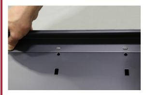
Align the shelf lip with the mounting holes on the front edge of the upgradable shelf. Use the M6x12 screws to attach the lip to the shelf, filling as many holes as possible.
