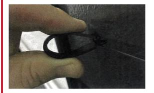
Insert notched ends of tool loop into slot horizontally.
