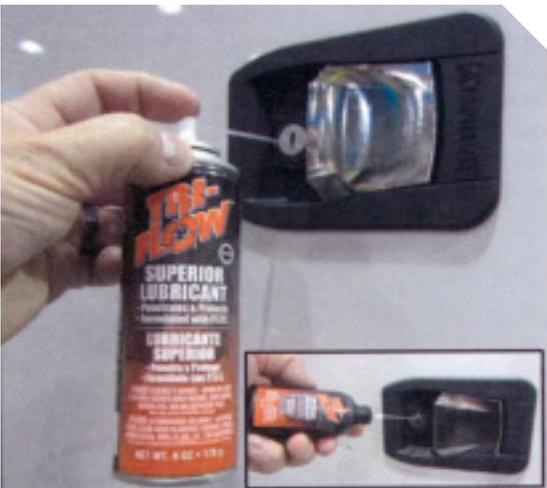
B. Lubricate Door Lock Cylinders
