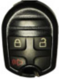
Knapheide PGN Series Bodies and Service Bodies equipped with the E-Lock system can be operated with the OEM Chassis Keyless Remote Fob **if the control module is wired to the OEM locking system.** With this system set-up, all Knapheide body doors lock or unlock in unison with the chassis cab doors.
