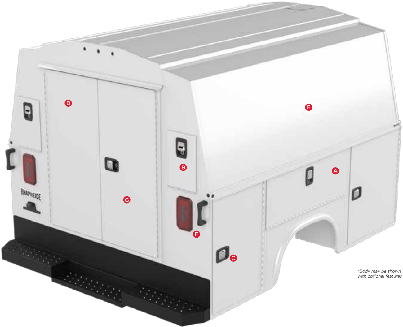
CARGO AREA AND CONDUIT CHUTE LENGTH 10.5' in 127" bodies 12.5' in 151" bodies
