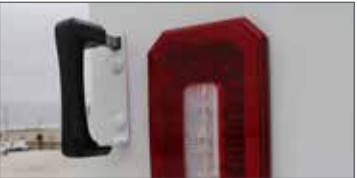
MASTER LOCKING SYSTEM for peace of mind — locks down all of the side compartments in one move
