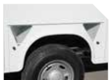
WHEEL CHOCK HOLDER - FENDER SKIRT
