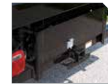
CLASS V RECEIVER HITCH
