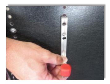
2. Position the wall hook in the desired location and fasten it to the end panel with the provided fasteners.
