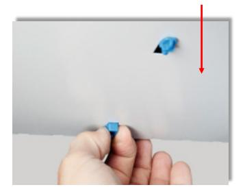
**4.** To remove the slide from the shelf, pinch the tabs at the rear of the BOXX slide from the underside of the shelf. Removal is the opposite of installation.
