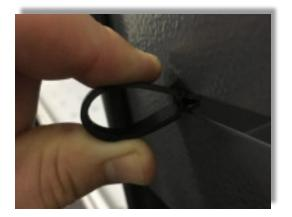
**2.** Insert notched ends of tool loop into slot horizontally.
