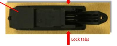
2. Installation is the reverse of removal. Insert the latch and apply slow pressure until the locking tabs click open.
