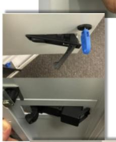
2. Installation is the reverse of removal. Insert the latch and apply slow pressure until the locking tabs click open.
