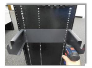
**3.** Secure the spool holder to the desired end panel in a horizontal position with the screws and nuts provided.
