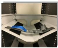
3. Install tank retaining straps through the provided slots on the front of the tank shelf.
