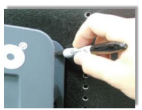
2. Level the hose holder and mark upper and lower hole locations to be drilled thru the Shelf Staxx end panel.
