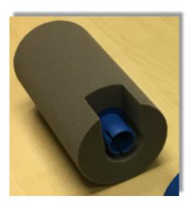
**6.** Addition of the foam stopper. The foam stopper is manufactured with a cutout on the side that attaches to the control arm. Fit the cutout end of the foam stopper into the control arm and apply pressure until the two pieces click together.
