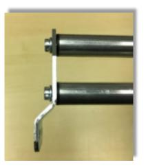
**3.** Attach the mounting brackets to the retention rods using the M6x25 screws (4). The rods will attach to the longer end of the bracket through the outer holes (center hole is not used). This end of the bracket will be oriented horizontally for installation.
