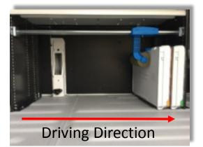
**NOTE:** The Case Clamp control arm will always point in the driving direction.
