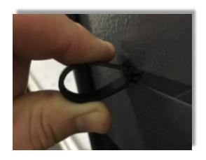
2. Insert notched ends of tool loop into slot horizontally.
