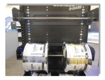
2. Installed wire spool holders shown.
