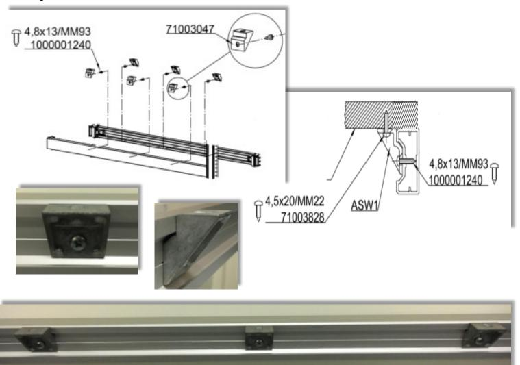
5. Set the worktop onto the frame supports and align it so that the worktop is flush with the front frame support. Attach the work top to the brackets using the 4.5x20 wood screws.
